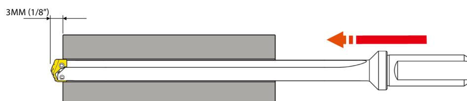
DEEP HOLE DRILLING - AT BREAKOUT
