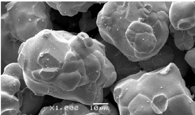
Traditional polycry stalline WC structure
